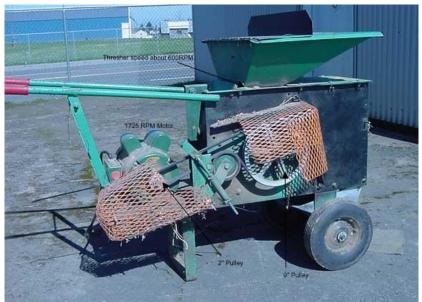
Figure 1. Bean thresher made from a modified chipper-mulcher at WSU Vancouver REU.
